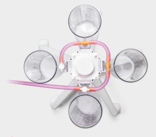
Complete the circuit with reinforced vacuum tubing and connect to the vacuum source.
