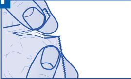
Gently tear open the package along the edges or corners. Handle with care to avoid puncturing the endocavity probe covers.
